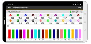
Our Insight $^{\text{TM}}$  for Mobile software allows you to reset, download, and analyze thermocouple operation on your tablet or smartphone via Bluetooth connection.
